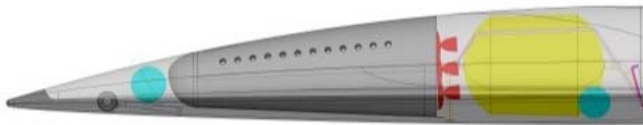
Figure 9: Potential location of the water tanks for the active cooling (side view)
