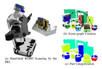
1. Overview of the process of scanning, segmenting and categorizing objects in clutter. In the final result cylinders are marked with blue, boxes with yellow, rectangular flat faces with cyan, and (half) spheres with red.
