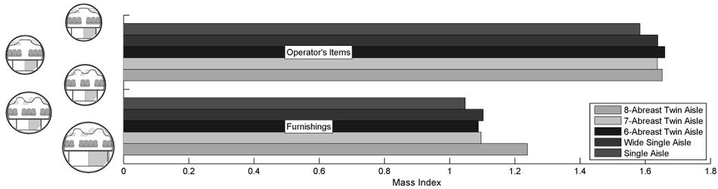
Figure 7: Fuselage secondary masses for different fuselage cross sections.
