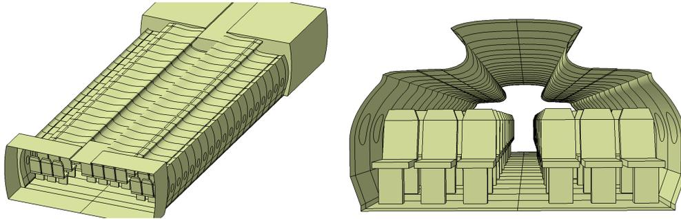
Figure 12: Screenshot of CATIA model for meshing. The geometry is watertight and allows direct meshing with little additional effort. Pictured is a part of an A380 cabin on the left, and a single aisle cabin on the right.
