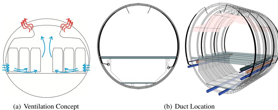
Figure 13: Concept of displacement ventilation and system ducting in fuselage section.
