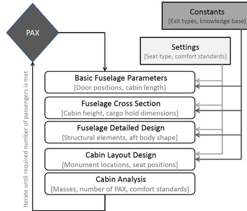
Figure 1: Process chart of the basic cabin and fuselage design.
