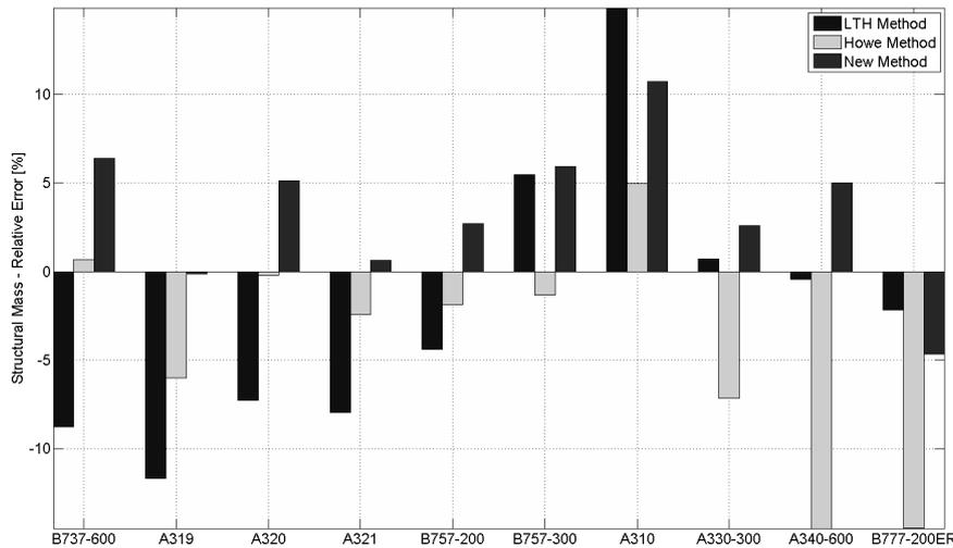
Figure 6: Comparison of different fuselage mass estimation methods. Shown is the relative deviation from the actual mass. The used method in the tool is called “New Method”, LTH and Howe Method refer to statistical methods.
