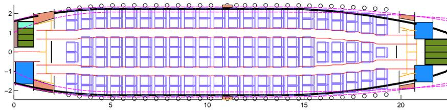
Figure 3: Layout of Passenger Accommodation (LOPA) of a 150-seat twin aisle.
