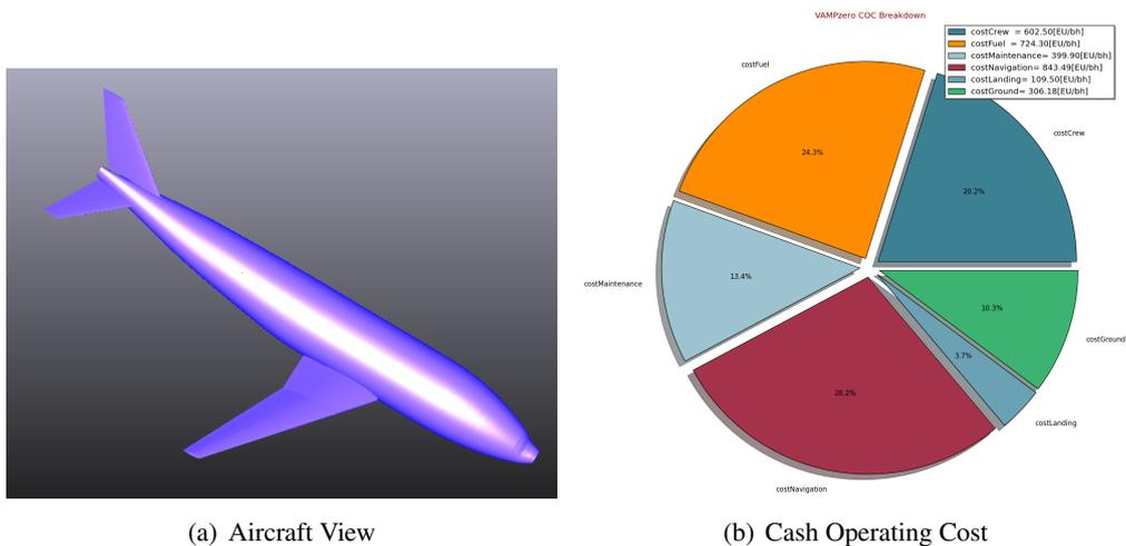
Figure 8: Result of sizing with VAMPzero. VAMPzero estimates all necessary components and delivers masses and cost of a reference mission, allowing the direct assessment of fuselage design decisions.
