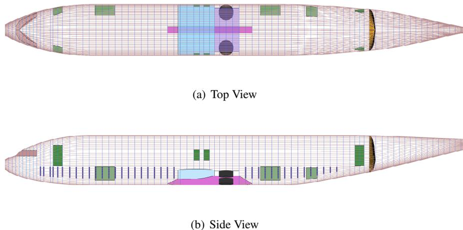
Figure 2: General structural arrangement of the fuselage. Note the doors and the center section with wing box and keel beam.
