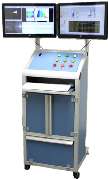
Fig. 5 Liquid feeding system developed at DLR with touch-screen controls and online diagnostic support
