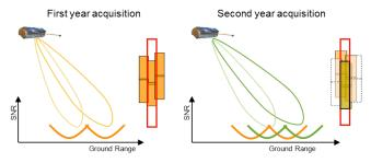
Figure 1: clapboard pattern and the scene overlap scheme: the second year is shifted by half the swath width to get a homogeneous quality.
