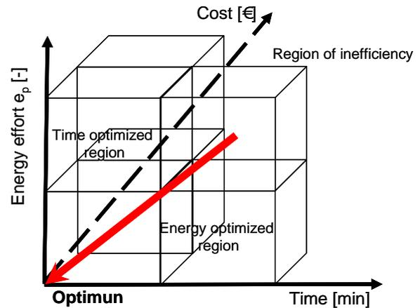
**Fig. 8: Transportation Efficiency Criterion**
