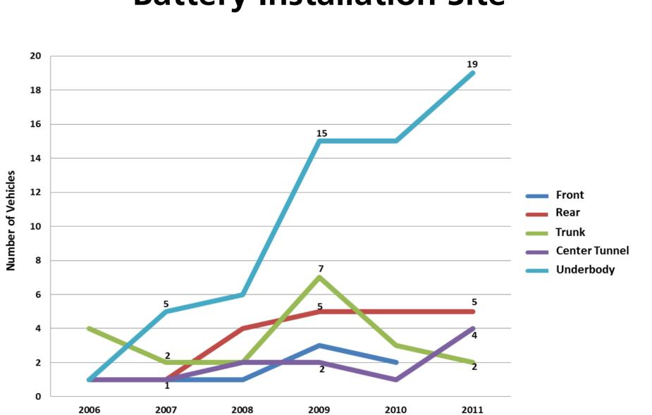
When investigating the installation site of the battery in Hybrid Electric Vehicles and Battery Electric vehicles, the underbody is by far the preferred location (light blue line).
