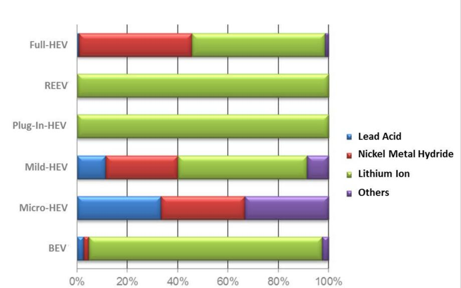
Lithium Ion (Li-Ion) battery technology (green) dominates Range Extended Electric Vehicles (REEV) and Plug-In Hybrid Electric Vehicles completely. For Battery Electric Vehicles (BEV). Li-Ion is the preferred battery technology for almost 95% of all analyzed vehicles.
