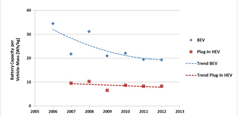
Over the years 2006-2012, the arithmetic mean of the specific battery capacity (Wh/kg) was decreasing. While the specific capacity of Plug-In HEVs (red line and dots) was reducing slightly, it was a significant process for BEVs (blue line and dots). The trend for BEVs suggests a capacity of around 20 Wh/kg vehicle mass over the next few years. For Plug-In HEVs, a capacity of around 8 Wh/kg vehicle mass seems to be probable.
