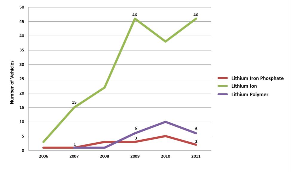
From 2006 to 2011 a strong increase in Li-lon battery technology (green line) can be investigated starting from only 3 prototype vehicles in 2006 to 46 in 2011. While the use of Lithium Iron Phosphate batteries (red line) remained constant in a range of 1 to 3 vehicles over time, Lithium Polymer batteries (purple line) were increasing from 2008 on, arriving at a peak of 10 vehicles in the year 2010.
