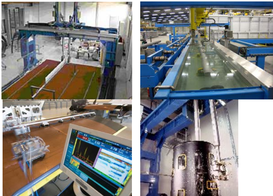
Figure 3 Examples for water coupled ultrasonic inspection (sources: National Composites Network, Premium Aerotec, IntelligeNDT, HPI)
