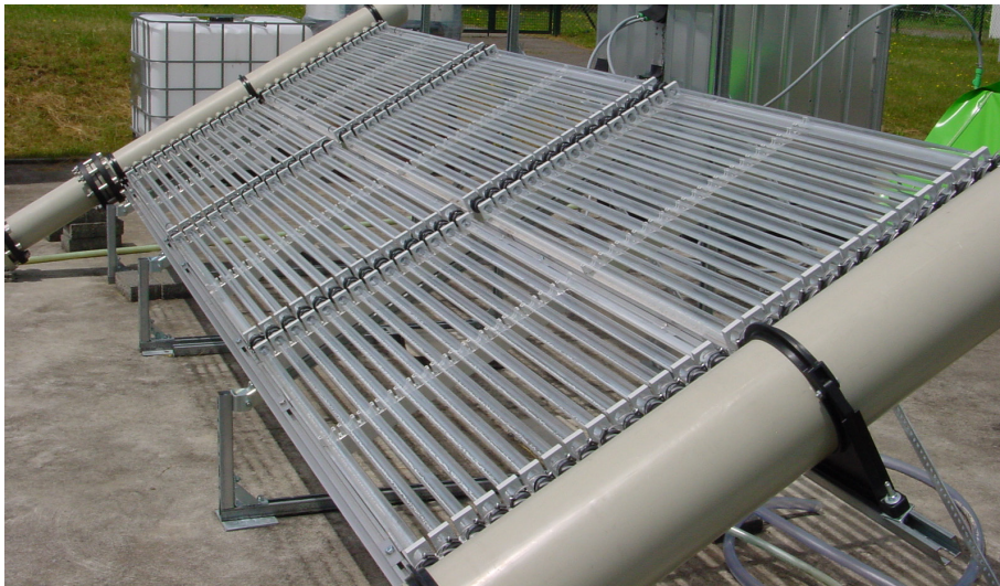
Fig. 1: Solar prototype reactor with non-concentrating tubular receiver modules at DLR, Cologne.
