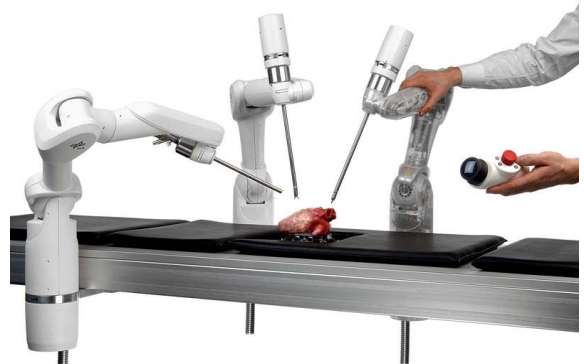
Fig. 1. Setup for using the DLR Medical robot.
