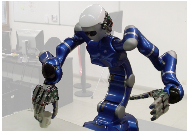
Fig. 1. The Justin robot learns to grasp and lift-up a mug by imitation. The reach-and-grasp movement is learned from human demonstrations. Latent-space dynamic motor primitives generalize the learned movement to new situations.
