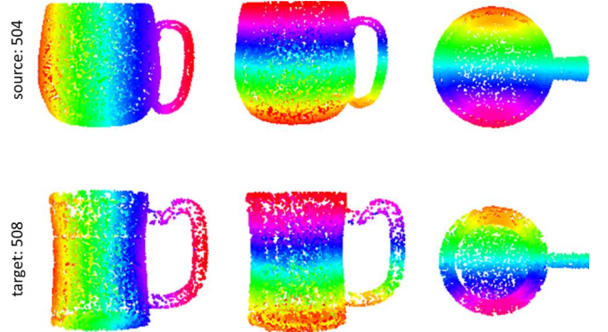
Fig. 4. Mug warping example. A dense set of surface points from the source mug (top row) and their mappings to the target mug (bottom row) are colored to code their three Cartesian source coordinates (three columns).
