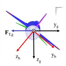
$\neg$  Control parameters :Initial values:Roll angle  $\phi$ =0°Pitch angle  $\Theta$ =5°Thrust=0 N $\eta_{arileron}$ =0° $\eta_{rudder}$ =0° $\eta_{HTP}$ =0°
