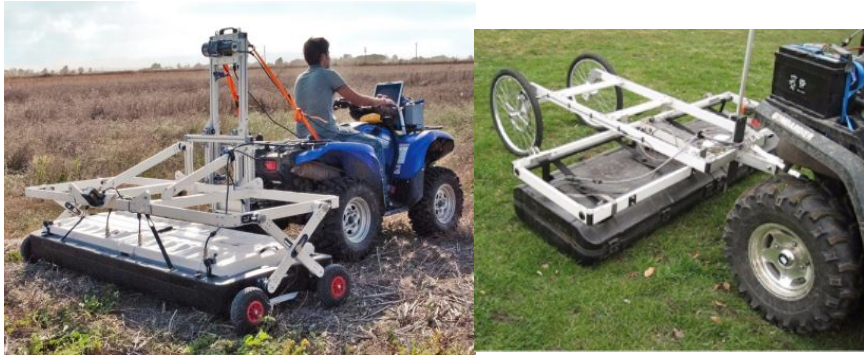
Figure 7. IDS' commercial GC GPR system STREAM-X (600 MHz) with different mechanical frames.
