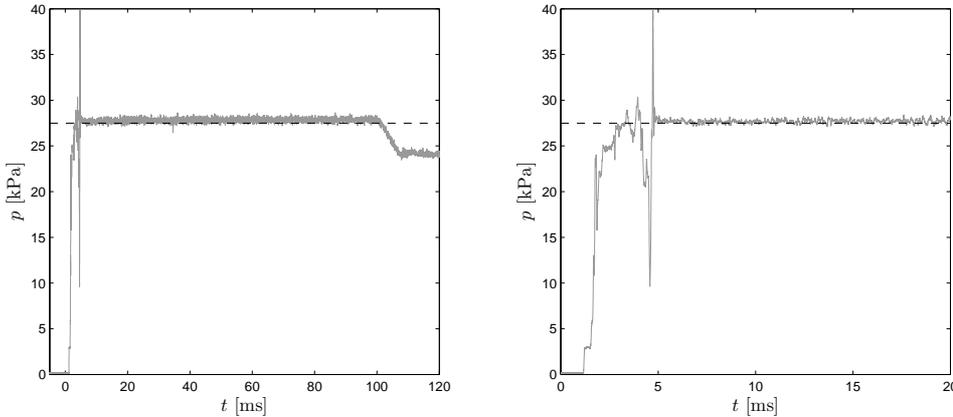
FIGURE 3. A sample Pitot pressure trace of the test-section flow: (left) showing the complete steady flow time of the tunnel; (right) showing the typical test duration employed in the present experiments. The dashed line in both plots indicates the theoretical Pitot pressure derived from the fill conditions.
