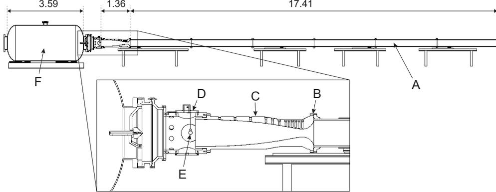
FIGURE 2. Schematic of the GALCIT Ludwieg tube facility (all dimensions are in metres) with a blow-up of the test-section region inset: (A) tube (internal diameter 0.298 m); (B) diaphragm holder; (C) converging-diverging Mach 4 nozzle (exit diameter 0.315 m); (D) test section (internal diameter 0.391 m); (E) suspended spheres; (F) dump tank.
