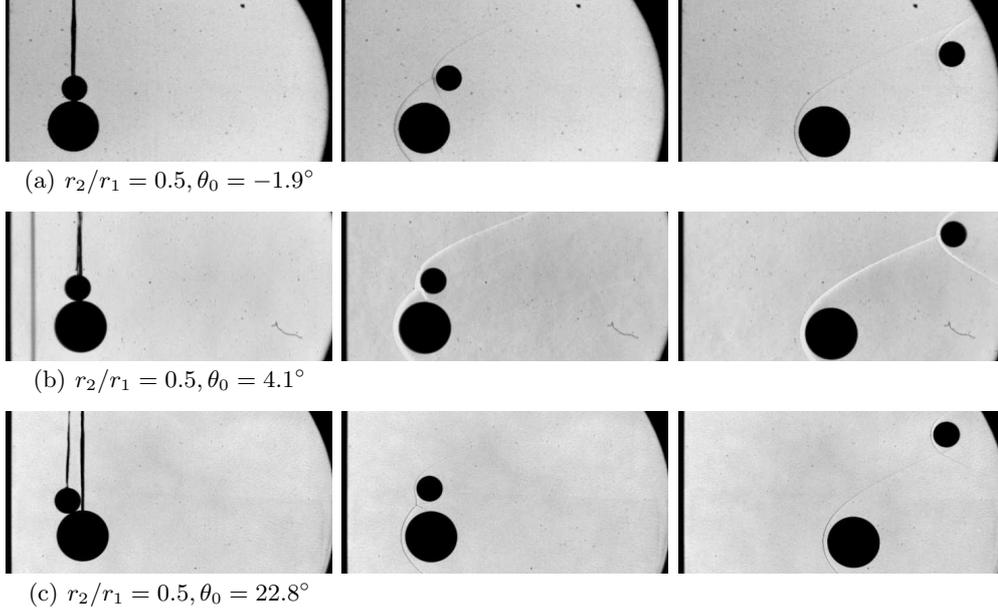
FIGURE 10. Separation behaviour for configurations with a constant radius ratio and varying initial alignment angles.
