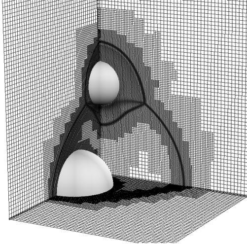
FIGURE 5. Cuts through part of the computational domain of setup 5 described in table 1 at  $t = T + 6.4151$ , visualising the mesh adaptation around the two bodies together with the shock waves on the cut planes. Two additional levels of refinement with  $l_{1,2} = 2$  are used.
