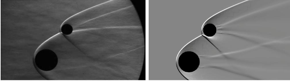
FIGURE 8. Comparison of experimentally and computationally (setup 5,  $t = T + 7.8367$ ) derived visualisations of the gradient of the fluid density in the  $y$ -direction. In the experimental image, the gradient has been effectively integrated through the fluid domain in the  $z$ -direction, while the computational image shows the gradient only on the central plane,  $z = 1$ .
