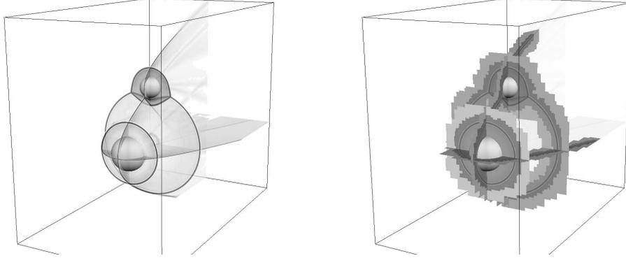
FIGURE 7. Schlieren plots of density (left) and domains of the two additional AMR levels (right), indicated by different grey scales, for  $t = T + 8.974$  in the setup 5 simulation.
