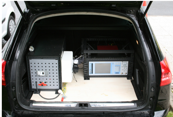
Figure 6: The OBU and power supply in the vehicle's trunk
