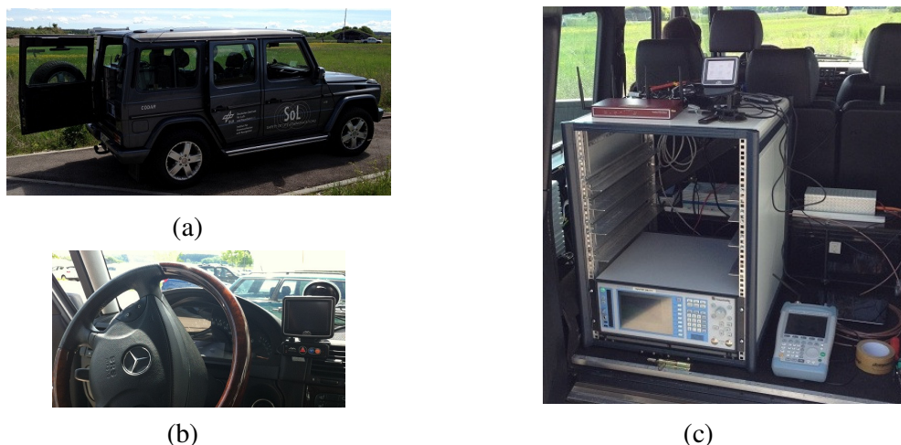
Figure 3: DLR Test vehicle (a), the driver HMI (b) and the rack containing the OBU (c)
