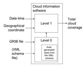
Figure 1. The structure of CIS.
