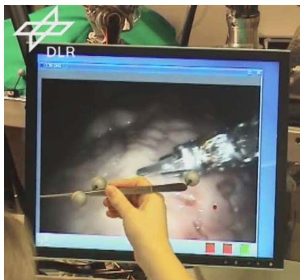
Fig. 8 The MiroSurge user interface: tracking of conventional instruments
