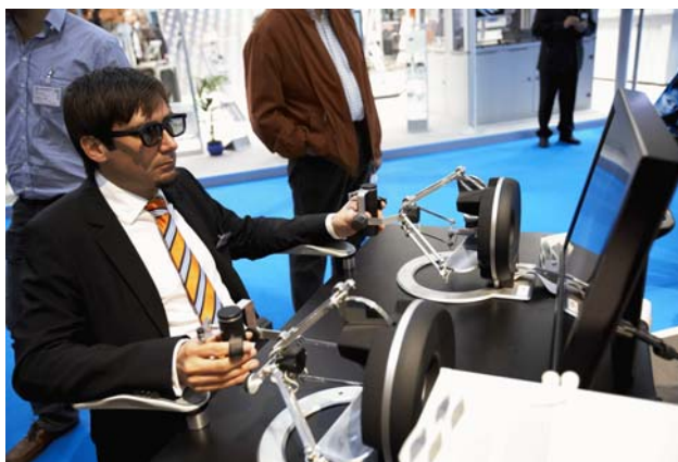
Fig. 7 The MiroSurge user interface: configuration with two Omega.7 devices and Miracube display
