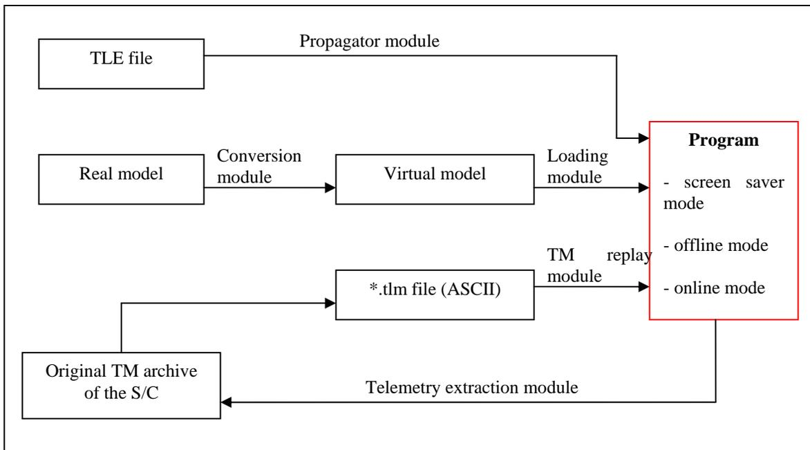
Figure 2 : General architecture of SatelliteSim tool
