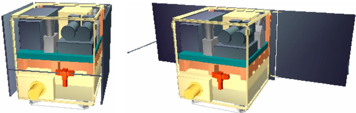
**Figure 4 : BIRD launch and flight configuration – industry drawing**
