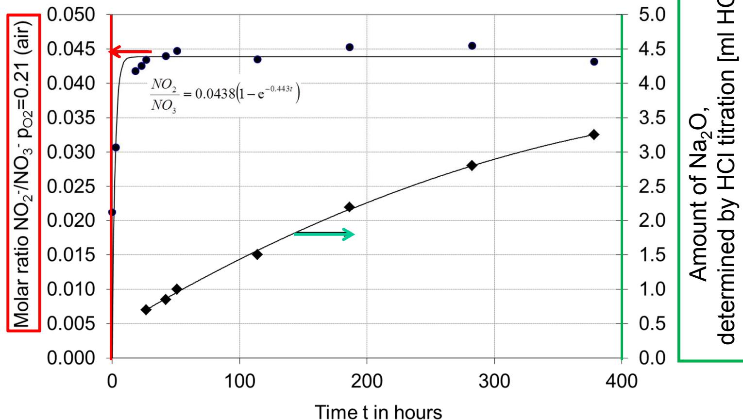
Solar Salt in synthetic air atmosphere in an open type system at 550 °C
