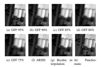
**Fig. 2**. GFF pan-sharpening (run with varying hf=0.95, 0.90, 0.85, 0.80, and 0.75) of WorldView-2 image is shown (green band is used for easier visual comparison). The quality of the ARSIS fusion (f) is comparable with the GFF 90% (b)
