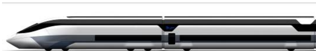
Figure 2: Side view showing the 21 m end car and a 20 m middle car
