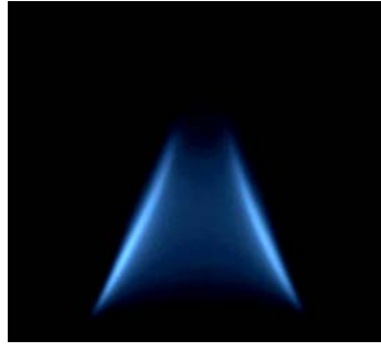
Fig. 4a. Premixed conical flame: \varphi = 1.5 ; open tip.
