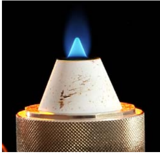
Fig. 3. Premixed conical flame: GtL/air, \varphi = 1.2 ; suitable for obtaining S_u .
