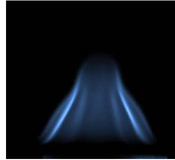
Fig. 4b. Premixed conical flame: \varphi = 1.55 ; wrinkled contour.
