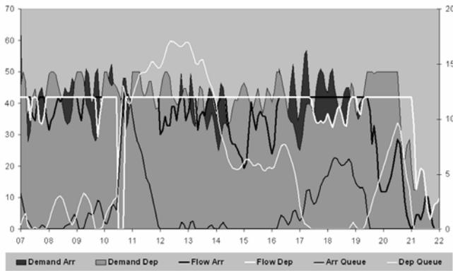
Figure 11. Flow trends (as Fig.7) – for case of runway system inhibition for 15 minutes (10:30-10:45) (non optimized reference).
