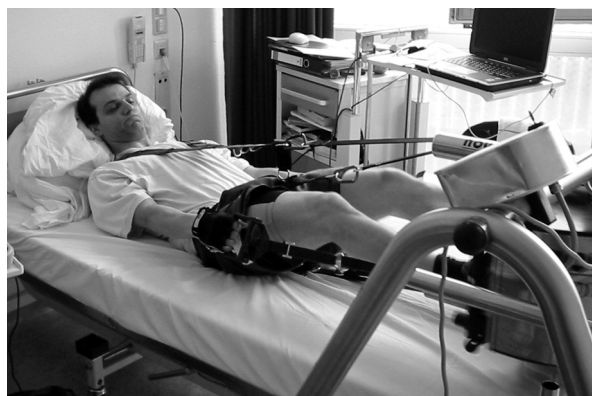
Fig. 1 - Resistive vibration exercise countermeasure during bed-rest. Subjects were required to perform leg exercises against a resistive force transmitted via belts at the waist and shoulders and via hand-grips. Vibratory stimuli in the legs are generated by rotation of the suspended platform around a vertically oriented axis. Axial loading of the spine occurs via the shoulder straps.
