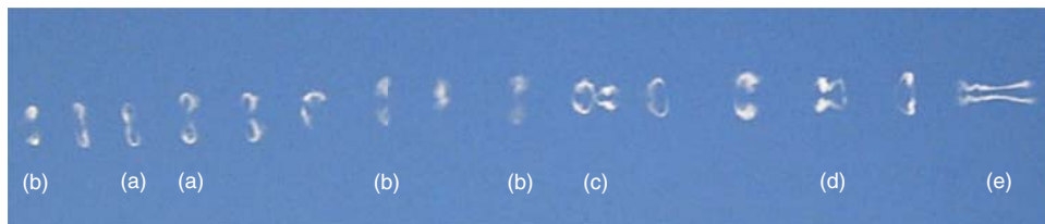
FIG. 7. (Color online) Photograph of a contrail featuring double vortex rings: flight direction from left to right. Photo taken from ground on November 16, 2006 at 8:53 by S. Lüke.
