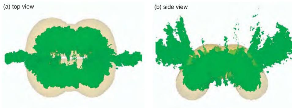
FIG. 21. (Color online) Passive tracer distribution (opaque, green) for the case \varepsilon^* = 0.01 and N^* = 0 at t^* = 7.0 with a control volume (transparent, orange) separating primary and secondary wakes: (a) top view, (b) side view.
