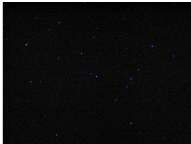
Fig. 11. Night sky image with the centroided stars in blue and the identified stars in red. (For interpretation of the references to color in this figure, the reader is referred to the web version of this article.)
