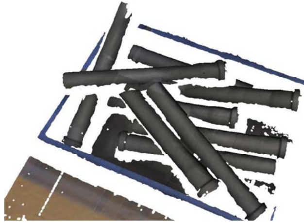
Fig. 11. Generated 3D model from a series of sweep scans over the filled bin.
