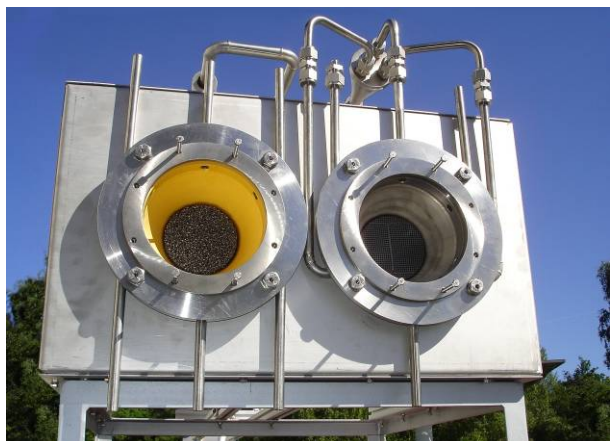
Figure 2: Solar reactor for decomposition of \text{H}_2\text{SO}_4
