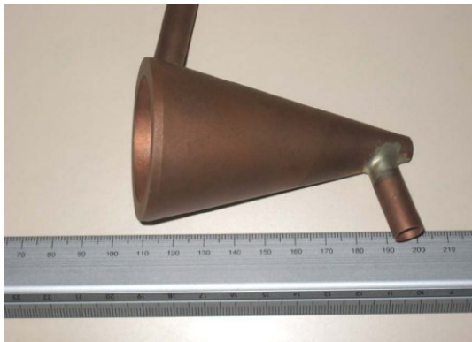
Fig. 1 Cavity of the new SunCatch II
