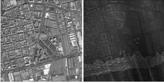
Figure 13: Detail of Terrassa testsite 1 km \times 1 km, left ortho image, right reference laser DSM points
