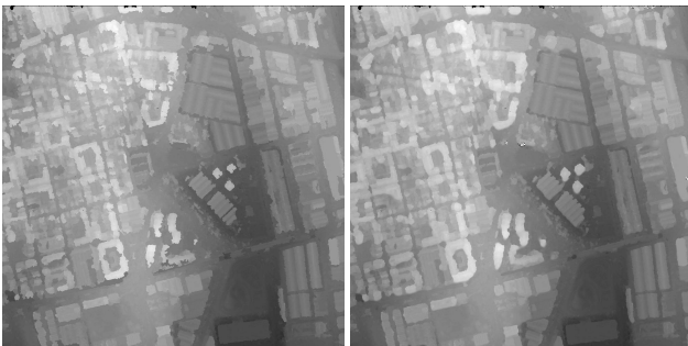
Figure 15: Detail of Terrassa testsite 1 km \times 1 km, left DSM filled with proposed method, right DSM filled using inverse distance weighted interpolation
