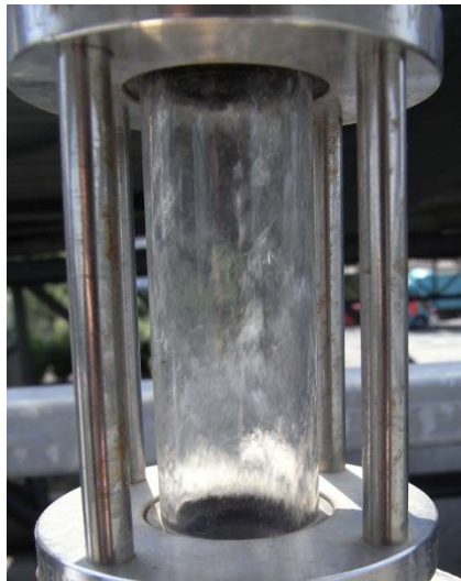
Fig. 3: Water steam mixture leaving the solar field downstream
