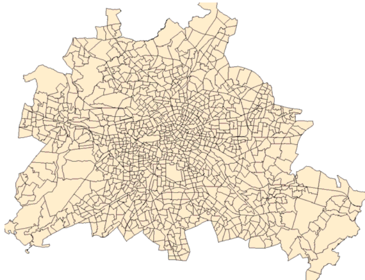
Fig. 2. Traffic zones used in the origin-destination matrix in the greater Berlin area
