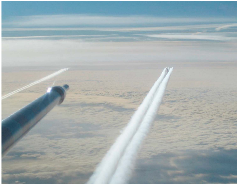
Figure 1. Probing contrails from two A340 aircraft on 19 November 2008 above Germany, photo taken from the cockpit of the DLR-Falcon.
