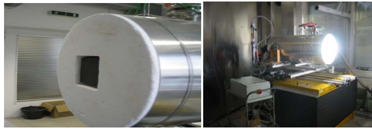
Fig. 2: Experimental set-up for absorber testing (left) and set-up during the operation (right)
