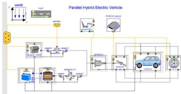
Figure 1: Exemplary Modelica vehicle model used for the simulation of a parallel hybrid.
