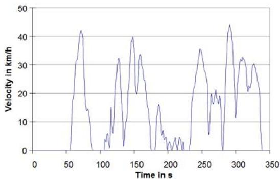
Figure 2: Segment of the newly developed driving cycle for delivery vehicles.
