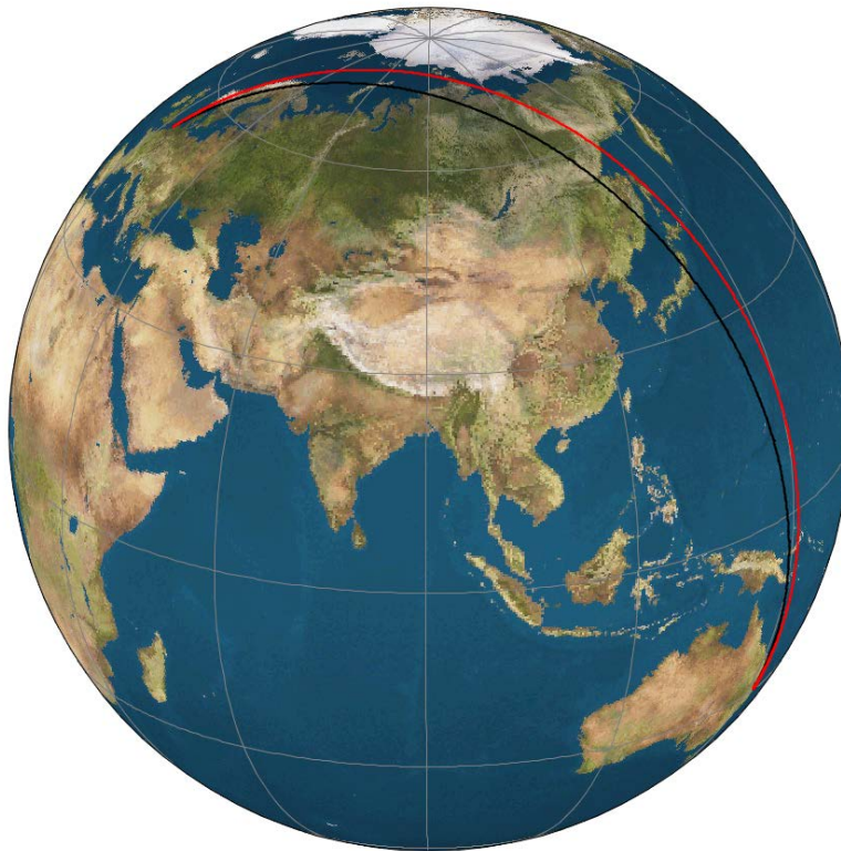
Figure 6. Groundtrack of ASTOS trajectory with initial azimuth released. The black line represents the skipping trajectory and the red line the no skipping trajectory.
