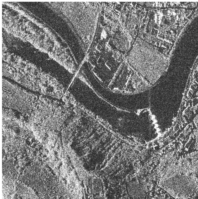
FIGURE 21 – Experiment with an actual SAR image. TerraSAR-X HR SL mode. Polarization HH, descending orbit, ground range resolution \sim 1.5 m, azimuth resolution \sim 1.1 m. Maribor, Slovenia, 29th of October 2008, 5 :01 :06 UTC.
