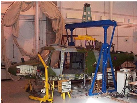
Figure 3 Test of Lynx Mk. 7 airframe at QinetiQ Farnborough
