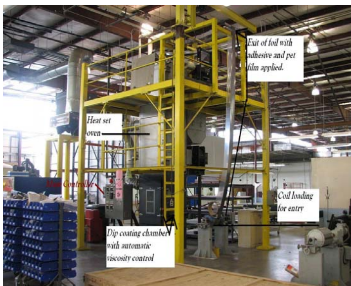
Fig. 3.6: MOD-3: Adhesive application.
