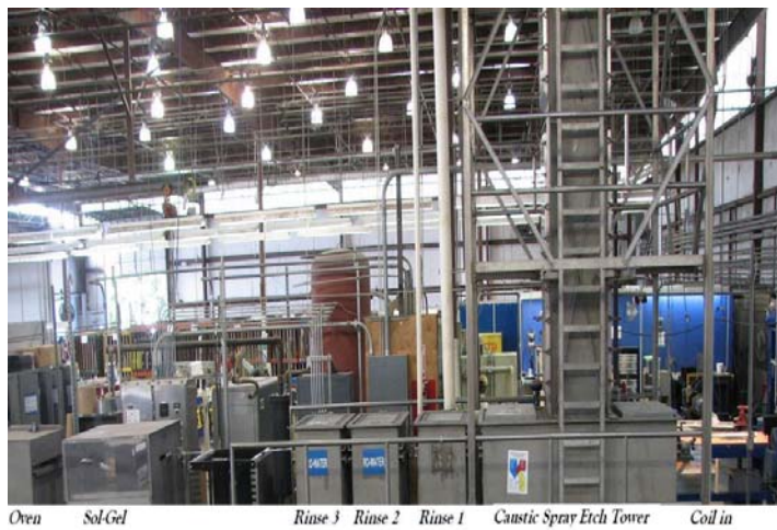
Fig. 3.5: MOD-2: etch and Sol-Gel.
