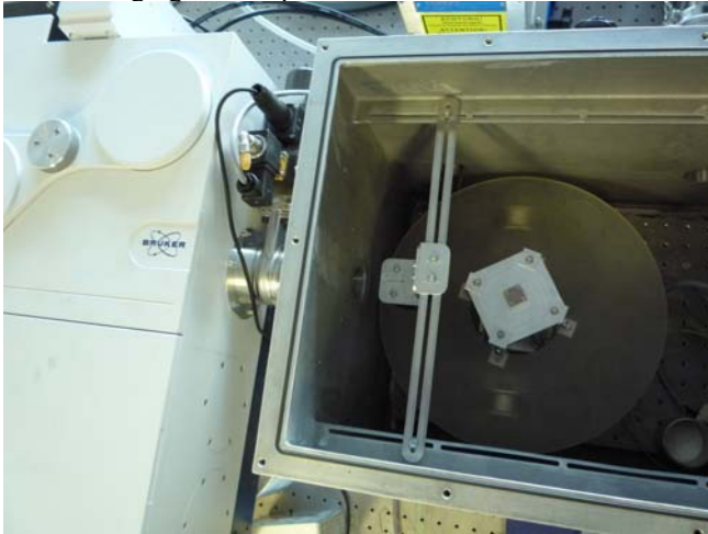
Figure 2. The planetary simulation chamber (top cover was removed)
