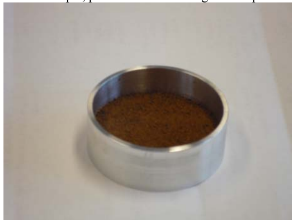
Figure 2: Cup with the JSC Mars-1 unsieved sample.
