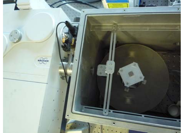
Figure 2: The planetary simulation chamber (top cover removed)
