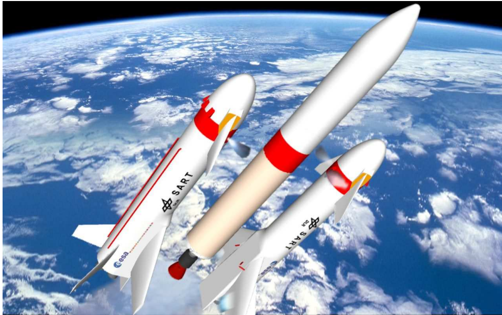
Figure 1: Artists impression of the separation of two attached reusable fly-back boosters from the Ariane 5 core stage
