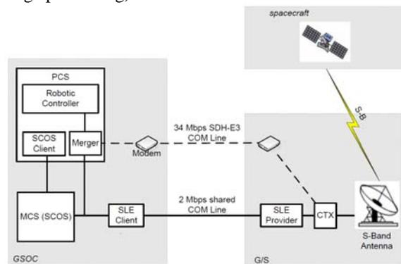
**Fig. 9:** Communication architecture to minimize delay time and jitter
