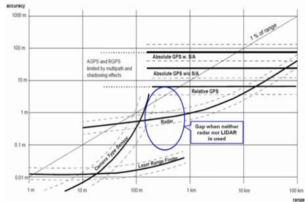
**Fig. 7:** Typical operational ranges of rendezvous sensors; the diagonal indicates the “1% rule” (diagram from FEHSE [10])
