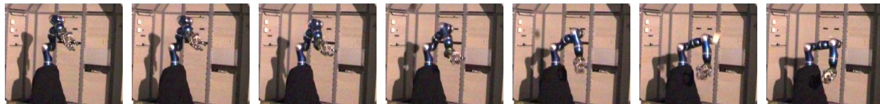
Fig. 10. Image sequence (from upper left to lower right) for “latest” mode catching with \Delta t = 120ms (same throw as in Fig. 9) and t \approx 0s for the first and t \approx t_{c,latest} + 20ms = 0.72s for the last image.
