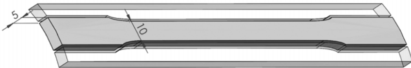
Figure 2: Waisted specimens for the measurement of tensile strength in axial direction with typical dimensions indicated were extracted from CMC pipes by water jet cutting. Similar specimens were extracted from plate material with orientations parallel and transverse to the original axial direction.
