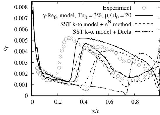
Fig. 3: Skin friction coefficient distribution for  $\alpha = -0.5^\circ$  and  $Re = 2$  Mio.
