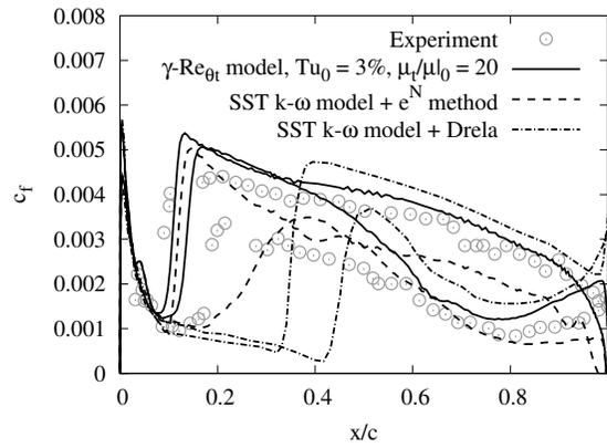
Fig. 4: Skin friction coefficient distribution for  $\alpha = -0.5^\circ$  and  $Re = 6$  Mio.
