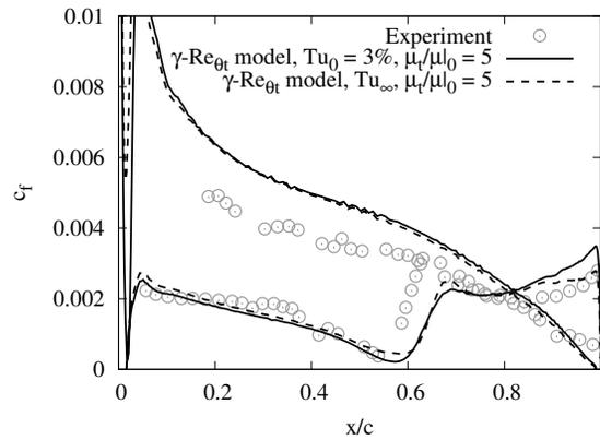
Fig. 5: Skin friction coefficient distribution for  $\alpha = 7.5^\circ$  and  $Re = 2$  Mio.
