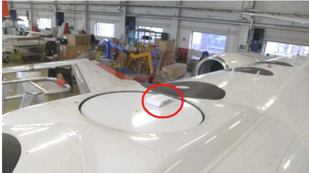
Figure 2: ANASTASIA navigation antenna mounted on top of test aircraft
