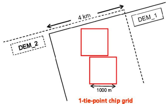
**Fig. 1: Tie-point chips in overlapping centers**
